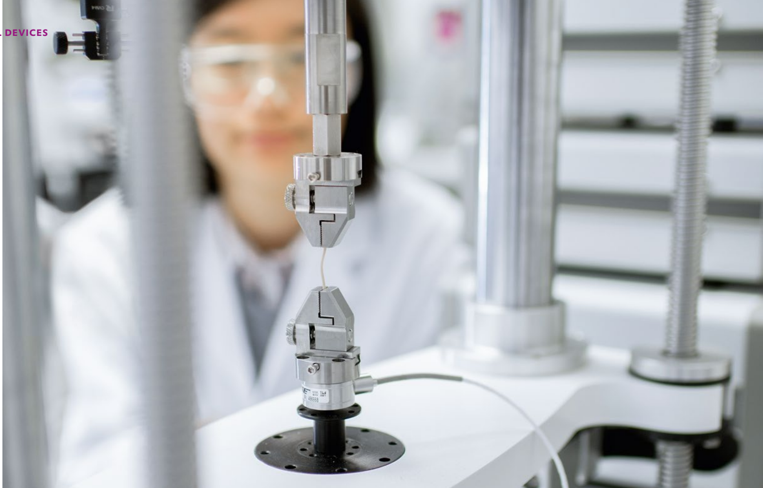
On the test bench: An injection molding prototype made of the newly developed composite material consisting of RESOMER® and hydroxylapatite
