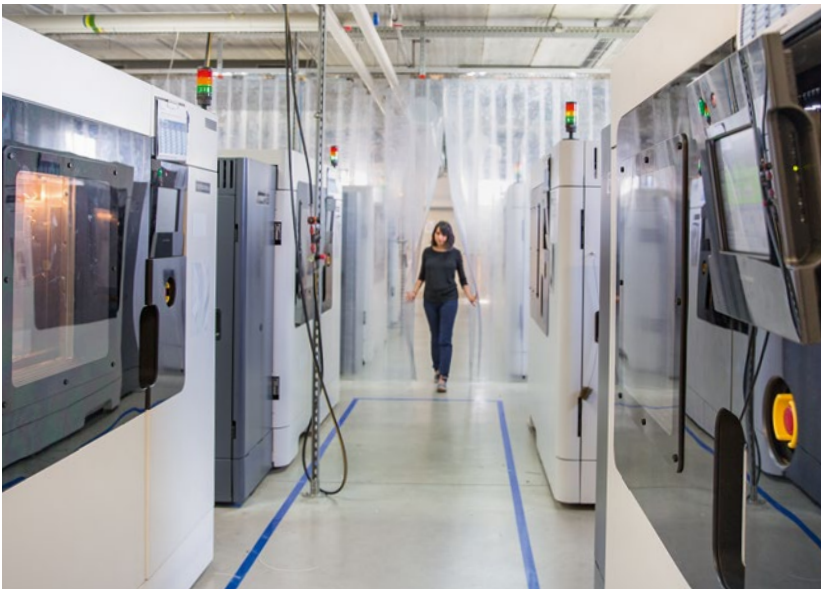
3D printing has to create added value, says Bart Van der Schueren (left photo). The selective laser sintering printers stand in long rows (bottom)
