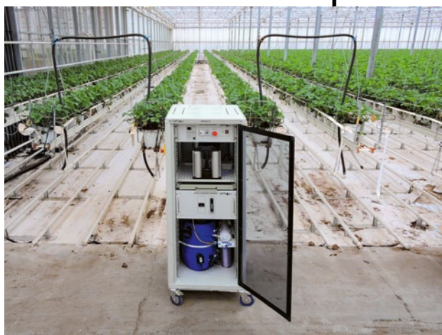
Far from the factory: Distributed H_2O_2 production in a greenhouse in Denmark
