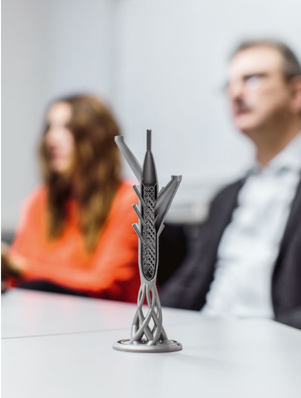
The interior of a demonstration piece printed from steel
