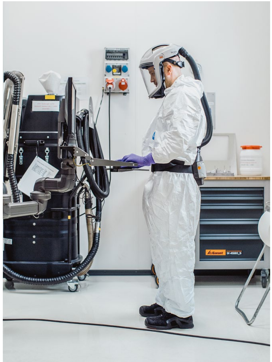
Plant operator David Fuchs wears a protective suit to fill a printer with metal powder
