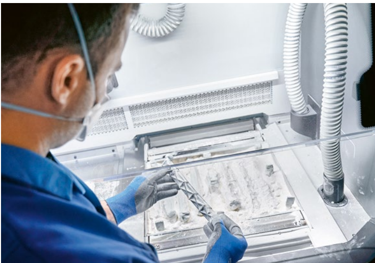
One of the methods that BMW uses for additive manufacturing is Multi Jet Fusion
