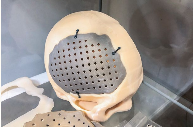
It's all in your head: Vestakeep® filaments are already used to make cranial, facial, and mandibular implants
