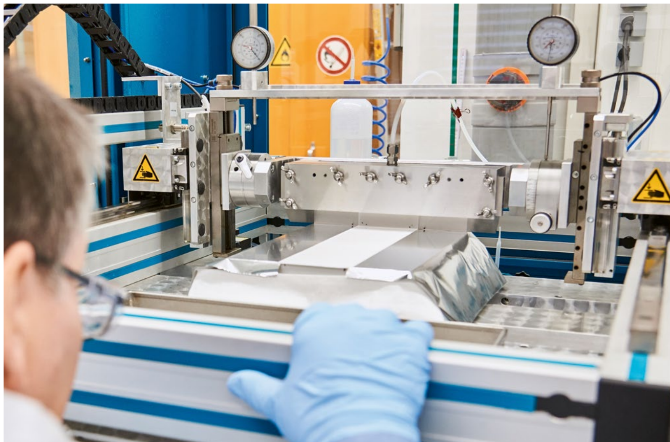
A fine piece of work At the Applied Technology unit in Hanau, Evonik demonstrates how separator films are provided with a ceramic coating
