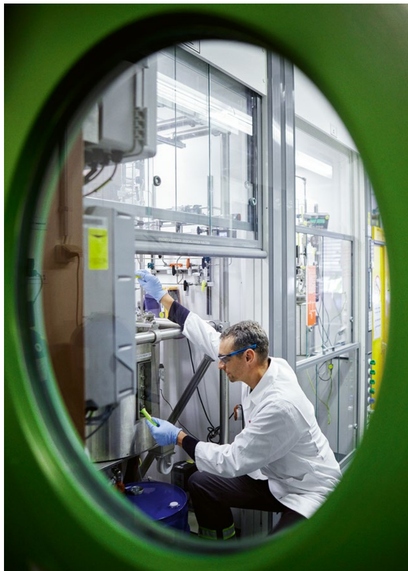
The 50-liter reactor is being filled with starting material. Michael Reuter checks the contents
