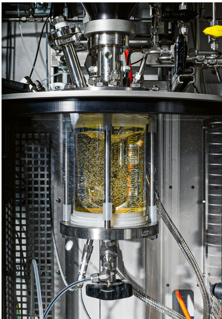
The one-liter glass reactor at the Evonik lab in Hanau is used for tests
