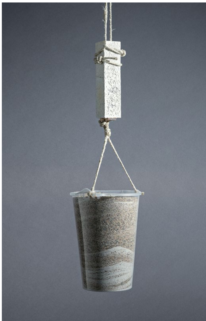
Long-term testing shows that cracks sealed by bacteria can withstand even extreme stresses
