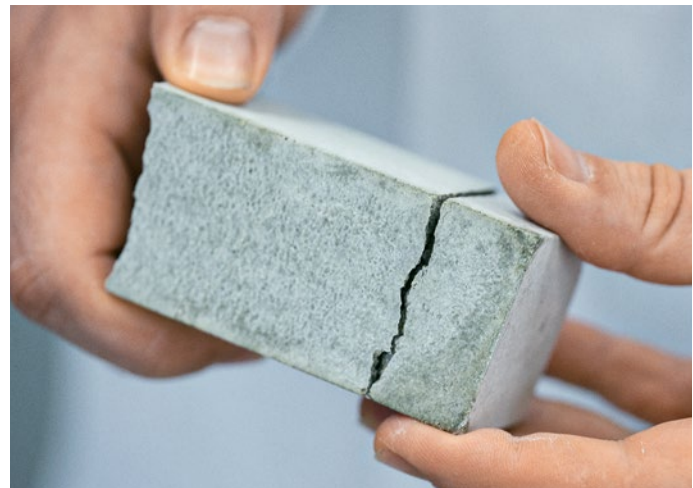
In the laboratory, the researchers create stress cracks that seal themselves automatically, thanks to WallCraft
