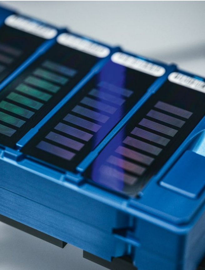
Evonik uses the infrastructure of the German Cancer Research Center in Heidelberg for some of its methylome analyses. This device reads out chips containing DNA samples
