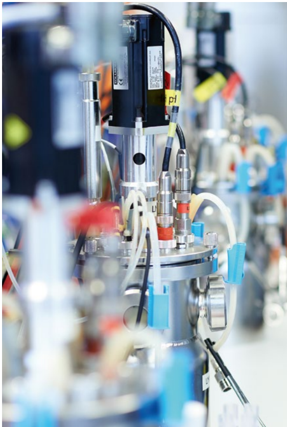
Small-scale fermenters play an important role in the development of fermentation processes
