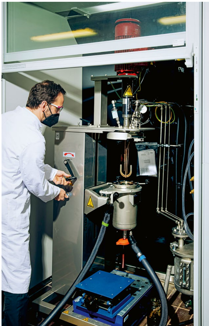
In order to fill his five-liter hydrolysis reactor with reactants, Michael Ferenz must turn the cranks vigorously
