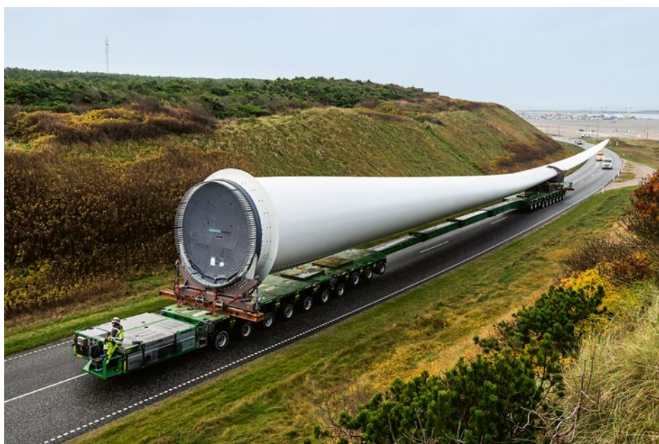
A great feat of logistics: A special transport vehicle is used to take the rotor blade of a Siemens wind turbine to its destination
