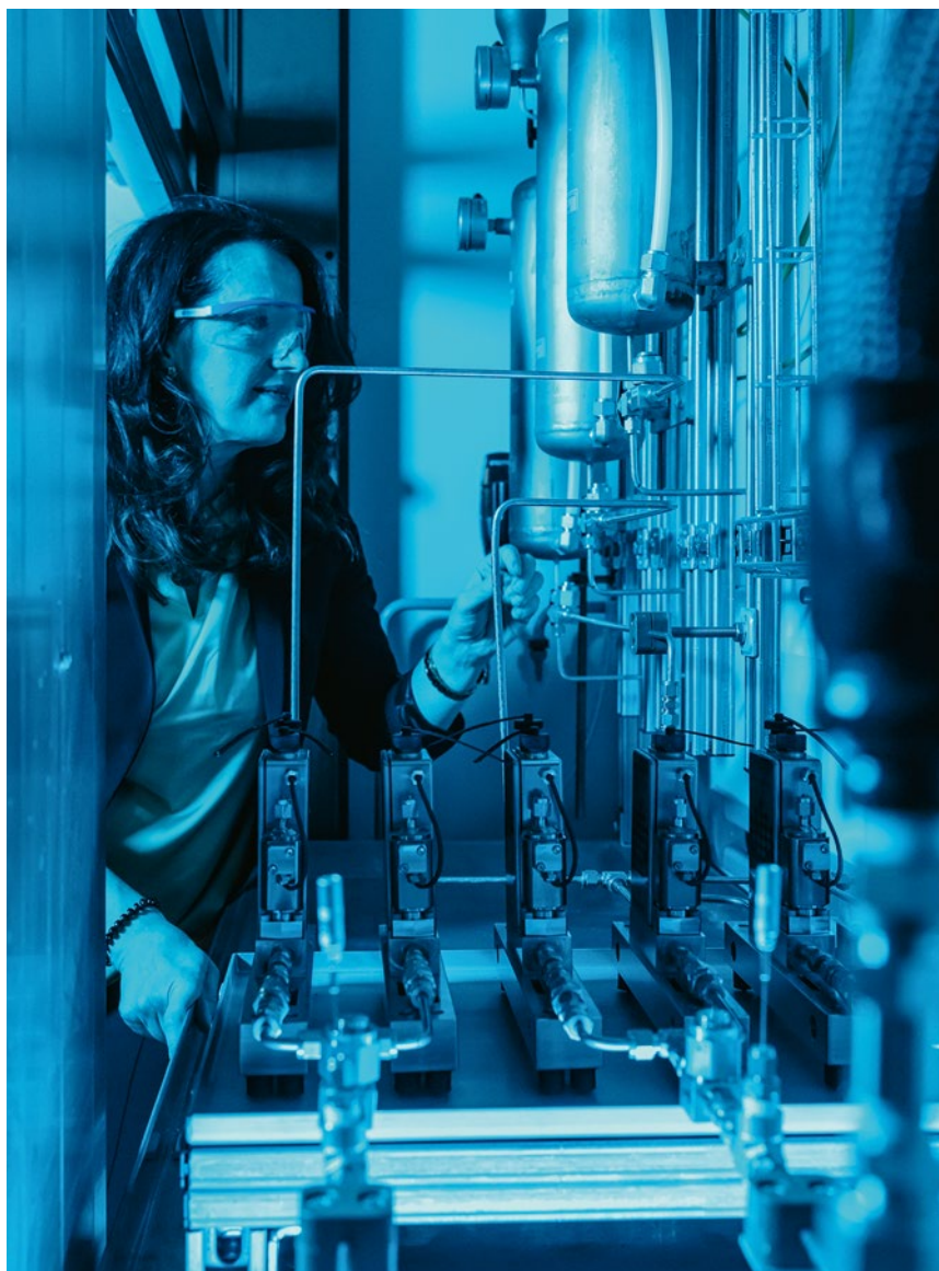
Senada Schaack inspects the ortho-lithiation apparatus. Plans call for the lines to soon lead to the first self-printed test reactor
