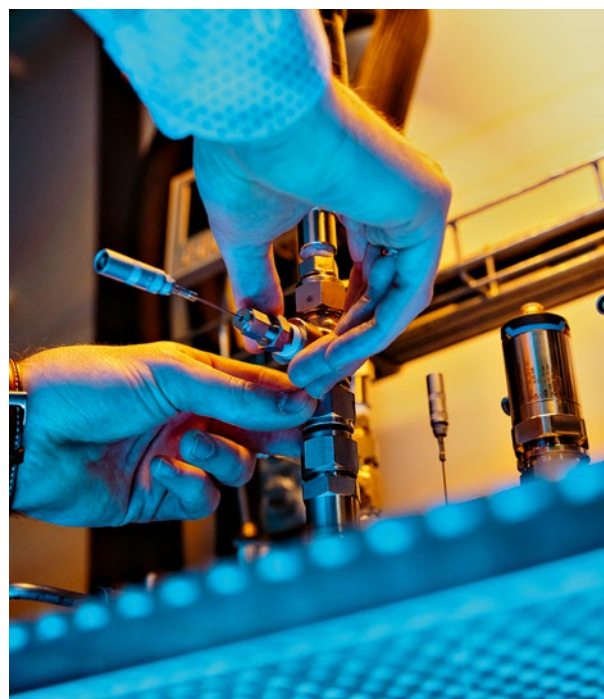
The heart of the test apparatus: The front horizontal tube (left) will soon be replaced by the 3D-printed version
