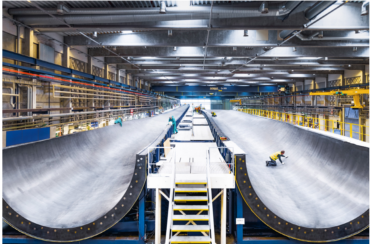
The molds used to make the rotors of large wind turbines are more than 100 meters long, as is the case here at Vestas in Denmark
