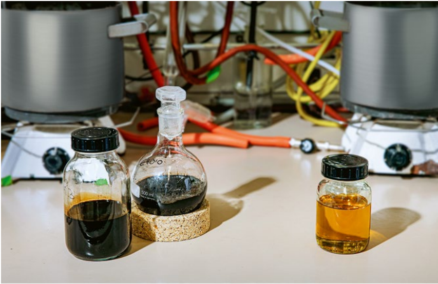
The hydrolysis produces a dark brown liquid in which the polyol and toluene diamine (TDA) are dissolved
