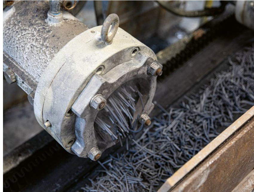
New strands of catalysts fall onto a conveyor belt to be dried.
