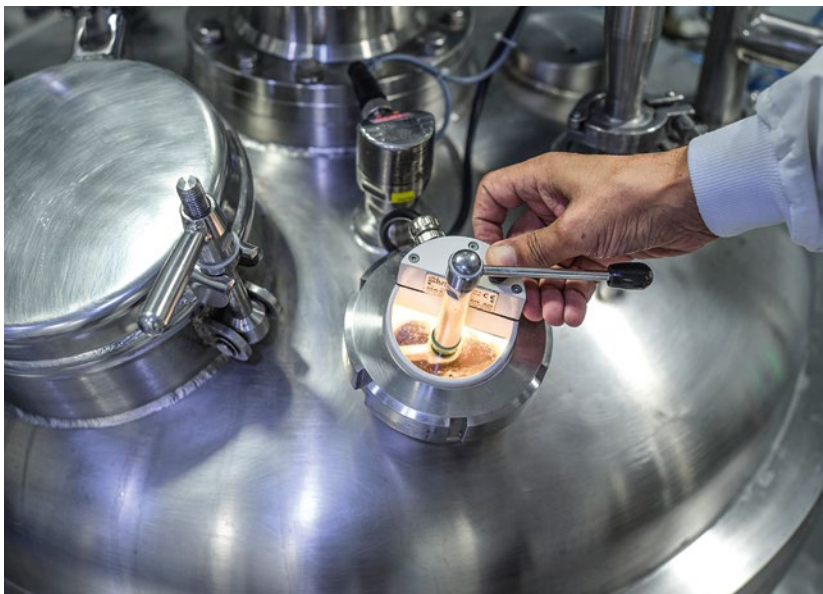
In the mixing reactor, active ingredients are mixed with the delivery system and other ingredients as well as with glycerin and water and then stirred for several hours to form a solution
