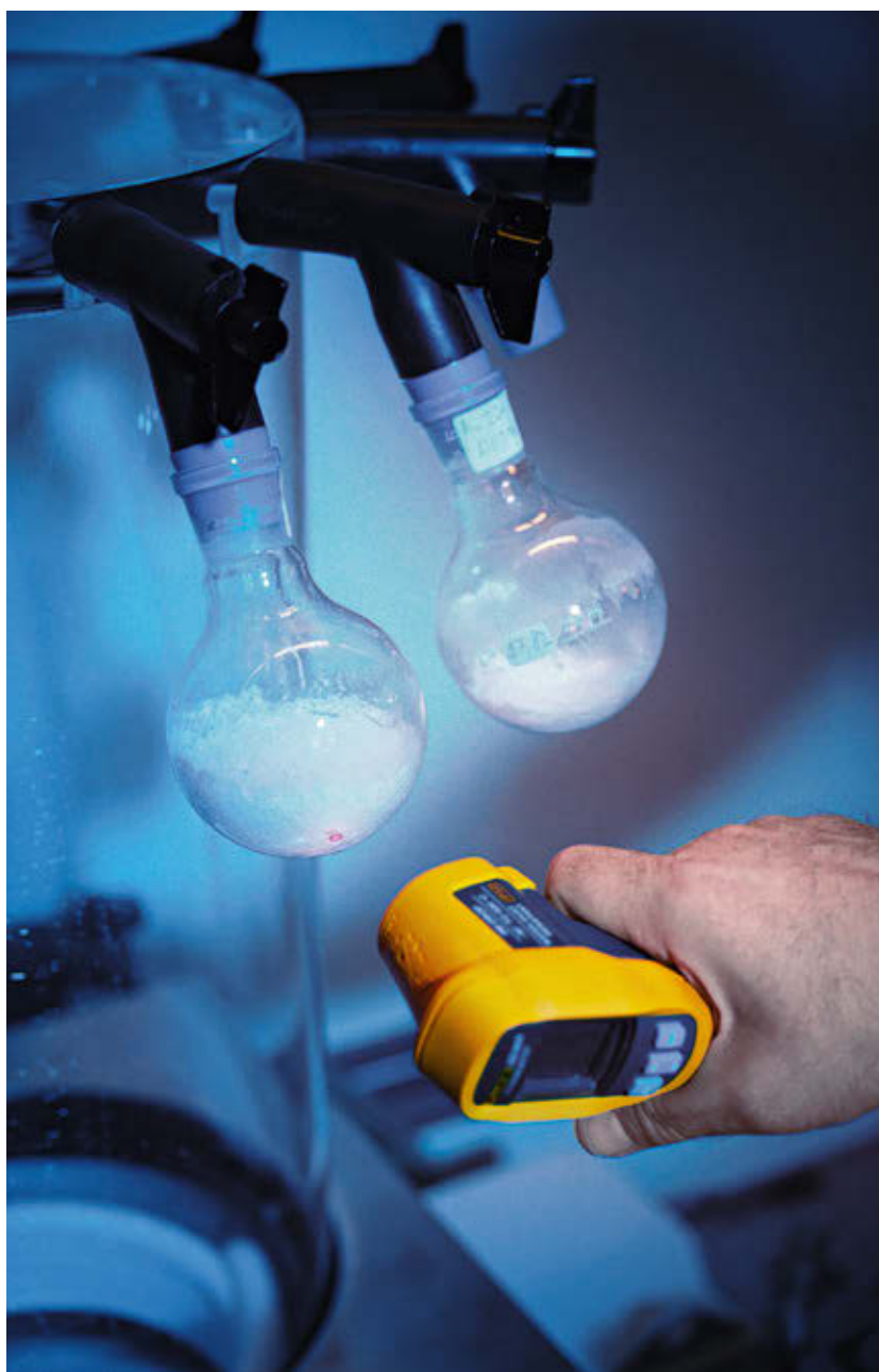
Freeze-drying the reaction solution produces the rPEG lipid in powder form
