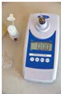
A peracetic acid (PAA) monitor is used to determine the amount of PAA residual remaining in the wastewater
