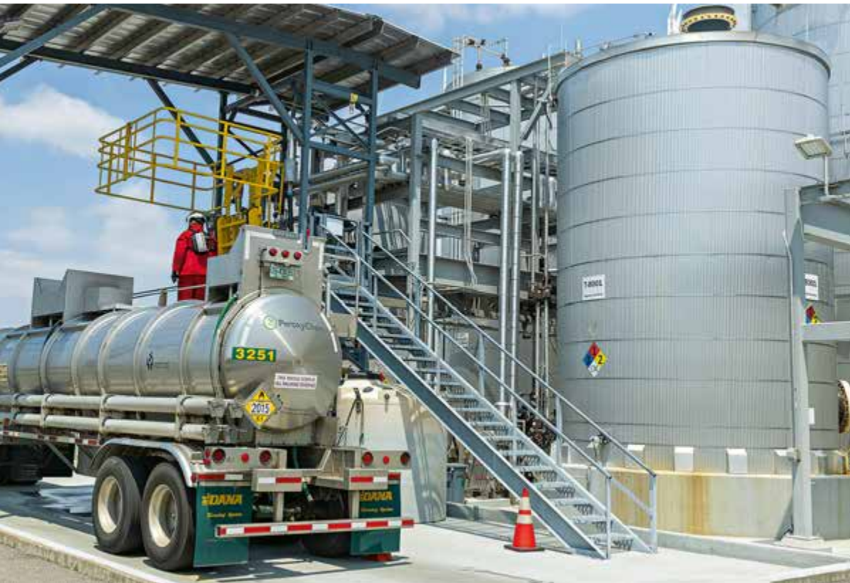
A worker prepares to offload hydrogen peroxide for the production of the disinfectant peracetic acid at Evonik’s Wolf River plant
