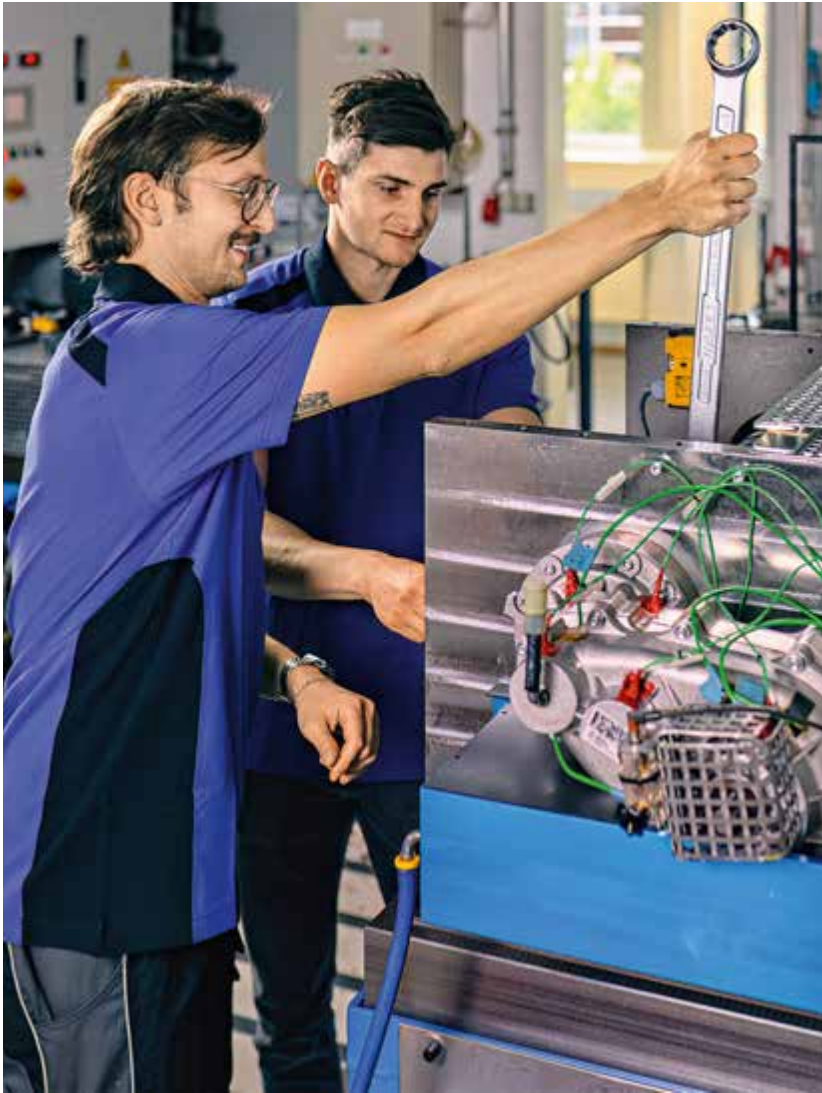
TUM doctoral candidates Nicolai Sprogies (left) and Stefan Reitschuster preset the torque on the transmission test bench in Garching
