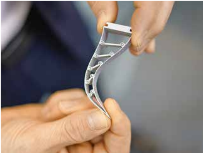
Ralf Düssel envisions diverse applications for plastic in the future—for example, for this 3D-printed component (left), which is used in robot grippers
