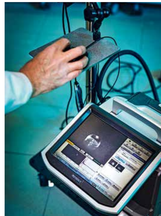
A camera is used in the laboratory to examine how drops land on a film and how they behave on it. Ideally, they stick and spread
