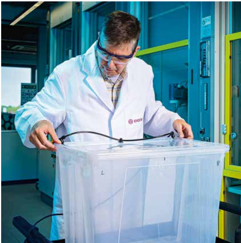
Research in a box: Laboratory technician Volker Klotzbach prepares a box to sprinkle water on plastic films coated with adjuvants
