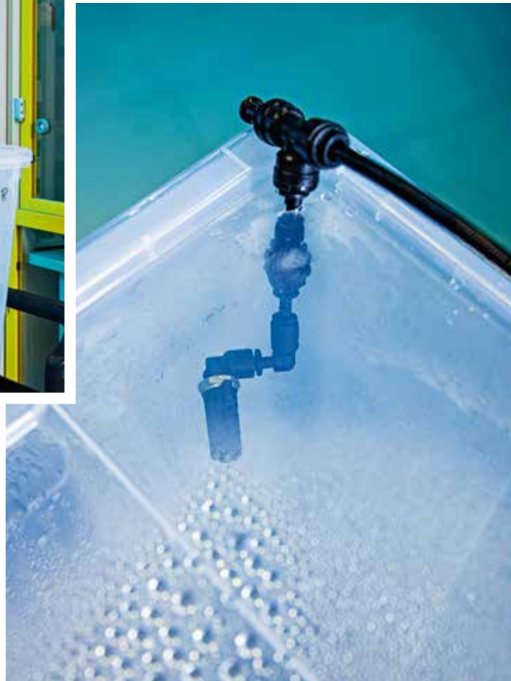
Research in a box: Laboratory technician Volker Klotzbach prepares a box to sprinkle water on plastic films coated with adjuvants
