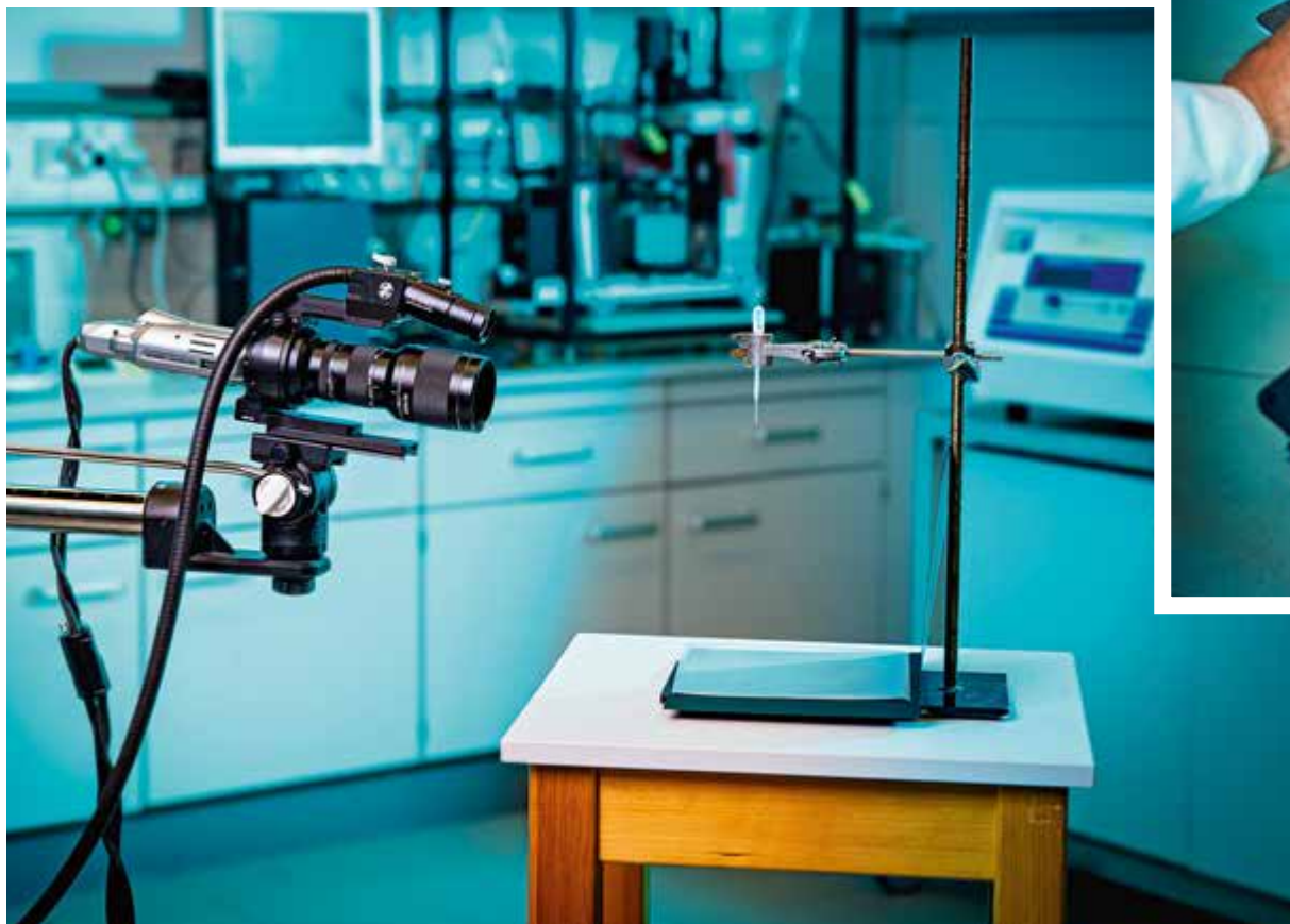
A camera is used in the laboratory to examine how drops land on a film and how they behave on it. Ideally, they stick and spread
