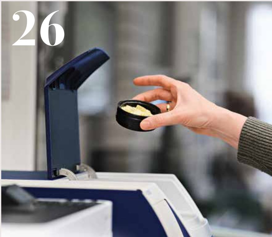
Near-infrared spectroscopy reveals the composition of the raw materials that are used to make compound animal feed at the Rothkötter production plant
