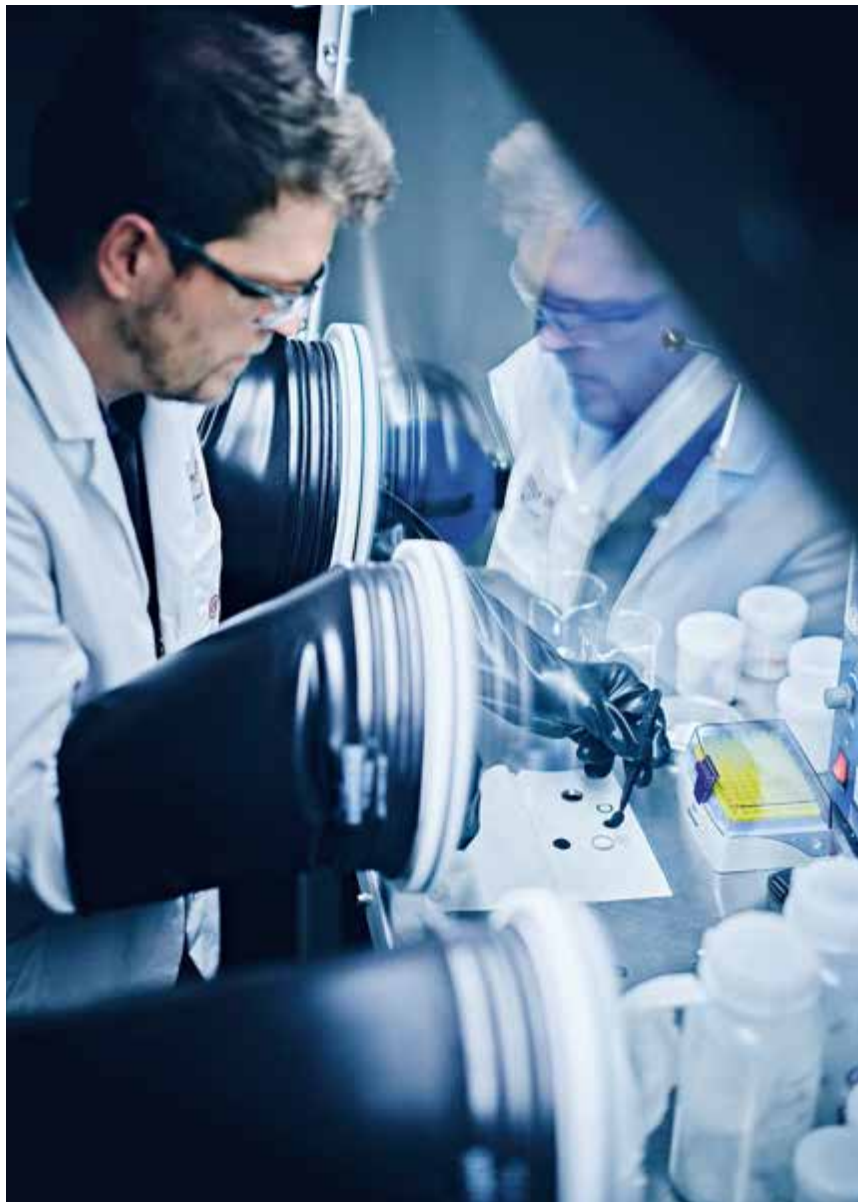
Dr. Frank Löffler builds the solid-state electrolytes into coin cells in order to test the materials' practical suitability
