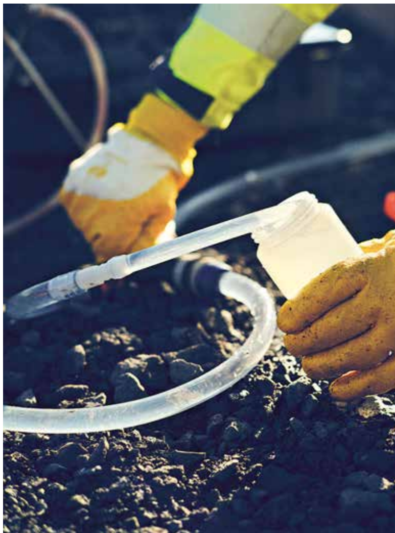
Water samples are regularly taken in Pioneer Park to document the progress of the remediation work
