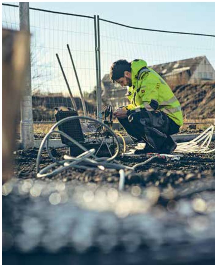
Water samples are regularly taken in Pioneer Park to document the progress of the remediation work
