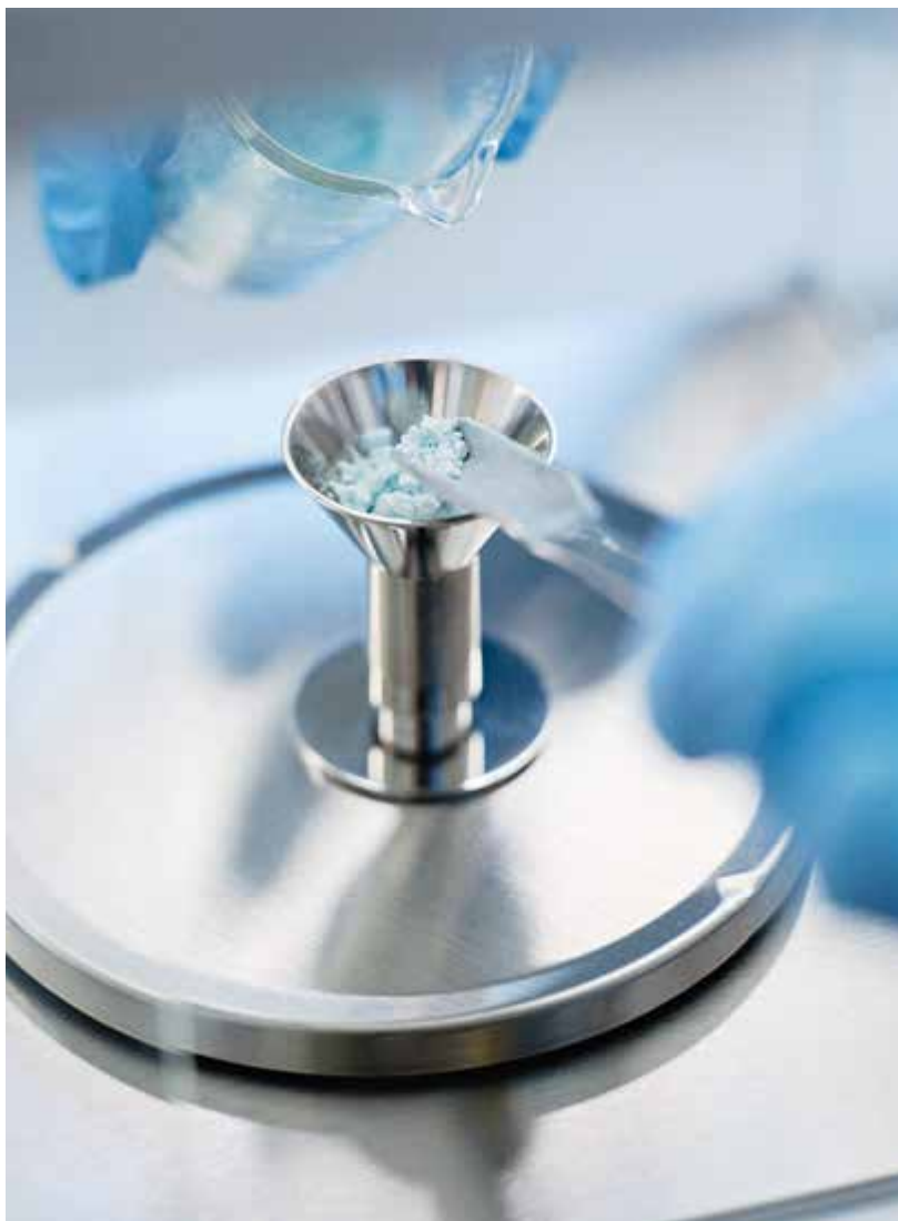
Chemistry lab technician Jessica Huppertz carries out the disintegration test with placebo-filled capsules
