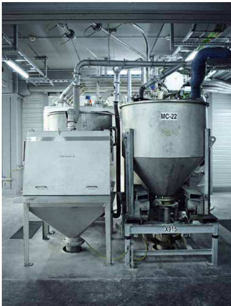
The raw polyamide is mixed with various additives in the compounding plant
