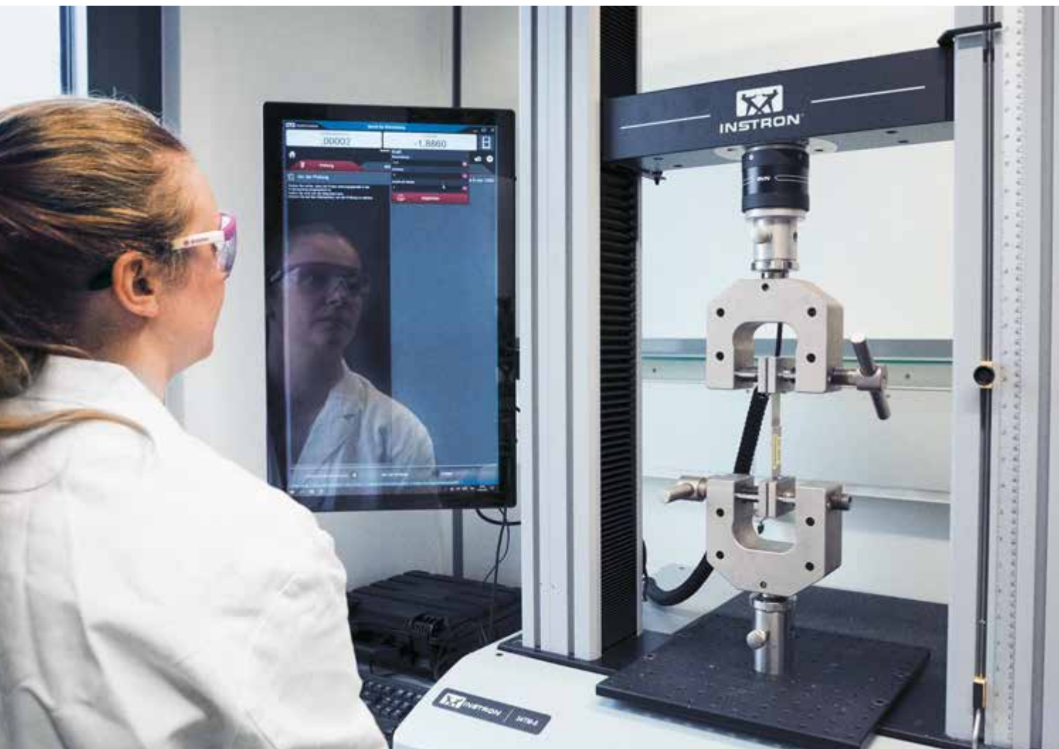
During tensile tests at the Essen Goldschmidt site, working student Anneke Henschel investigates how effective the debonding solution is compared to conventional adhesives
