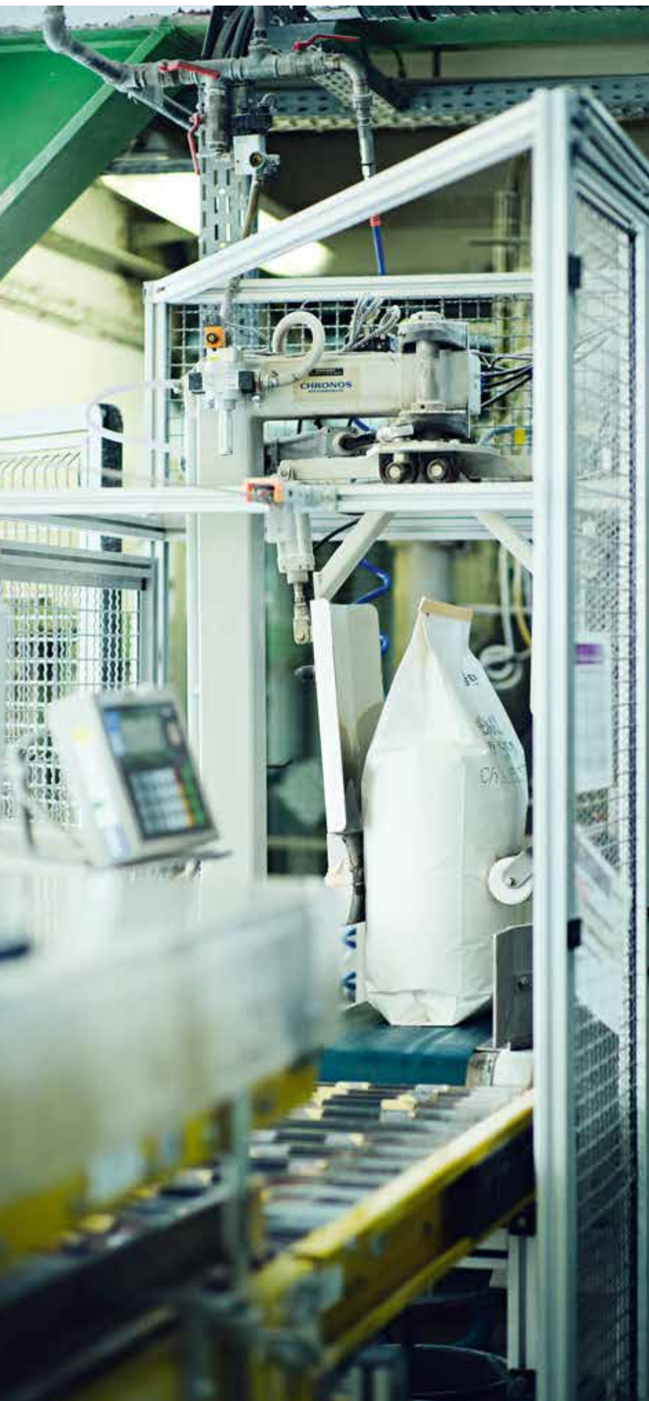
TEGO® Res 1100 is filled into bags fully automatically in Darmstadt
