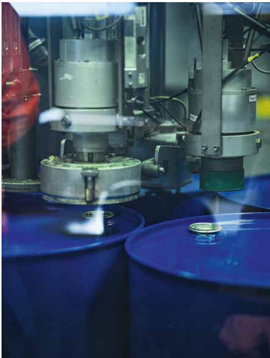
Fully automatic filling: The lids of the transport drums are positioned and screwed down under computer control. A filling nozzle is then inserted into the hole and the liquid silane mixture is pumped into the drum
