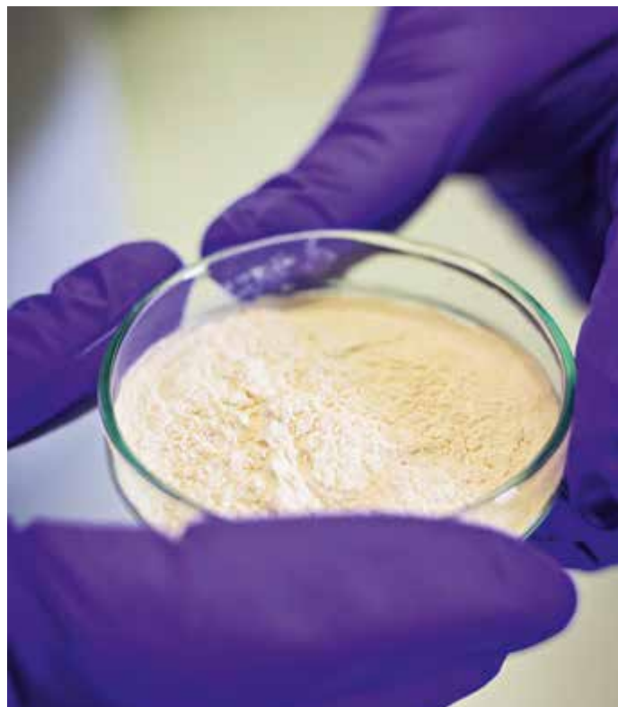
In the Evonik Fermas laboratory, lab technician Kristina Gabonova checks the purity of the protein using liquid chromatography (left). After drying, a white powder—spider silk protein—remains (above)
