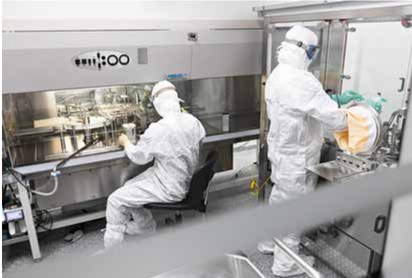
Fully suited operators monitor vial fill stations for LNPs in the clean room of Vancouver Labs. Phase 1 and 2 clinical production runs take place in Vancouver, while larger Phase 3 and commercial manufacturing are conducted at Evonik's site in Birmingham, Alabama
