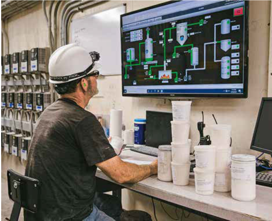
The production process in Little Rock is continuously monitored and product quality is ensured by taking samples
