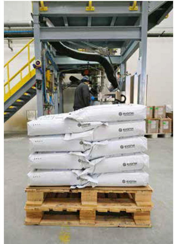
The plates with the spores are crumbled by a machine, mixed with excipients, and filled into bags for transport to customers
