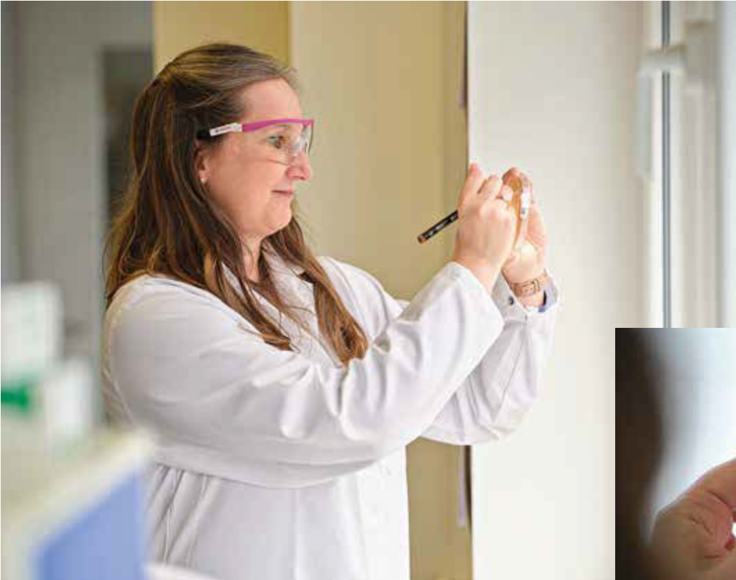
Microbiologist Stella Molck counts the bacterial colonies on an agar plate in the laboratory. Under good conditions and warmth, each spore in the sample outgrows into a visible colony containing around one million bacteria
