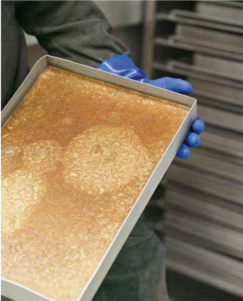
After fermentation, the biomass is centrifuged, shock-frozen into plates, and freeze-dried
