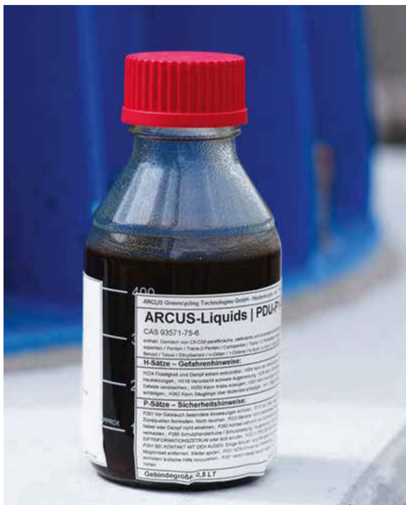
The result of pyrolysis is an oil that can be used in the synthesis of plastic polymers
