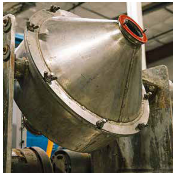
In drums like these, catalytically active metals are distributed on an adsorption material that can separate undesirable substances from the starting material and bind them
