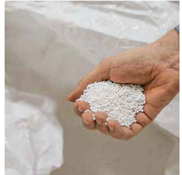
The adsorbents are white when freshly manufactured. They will turn gray during their use purifying pyrolysis oil
