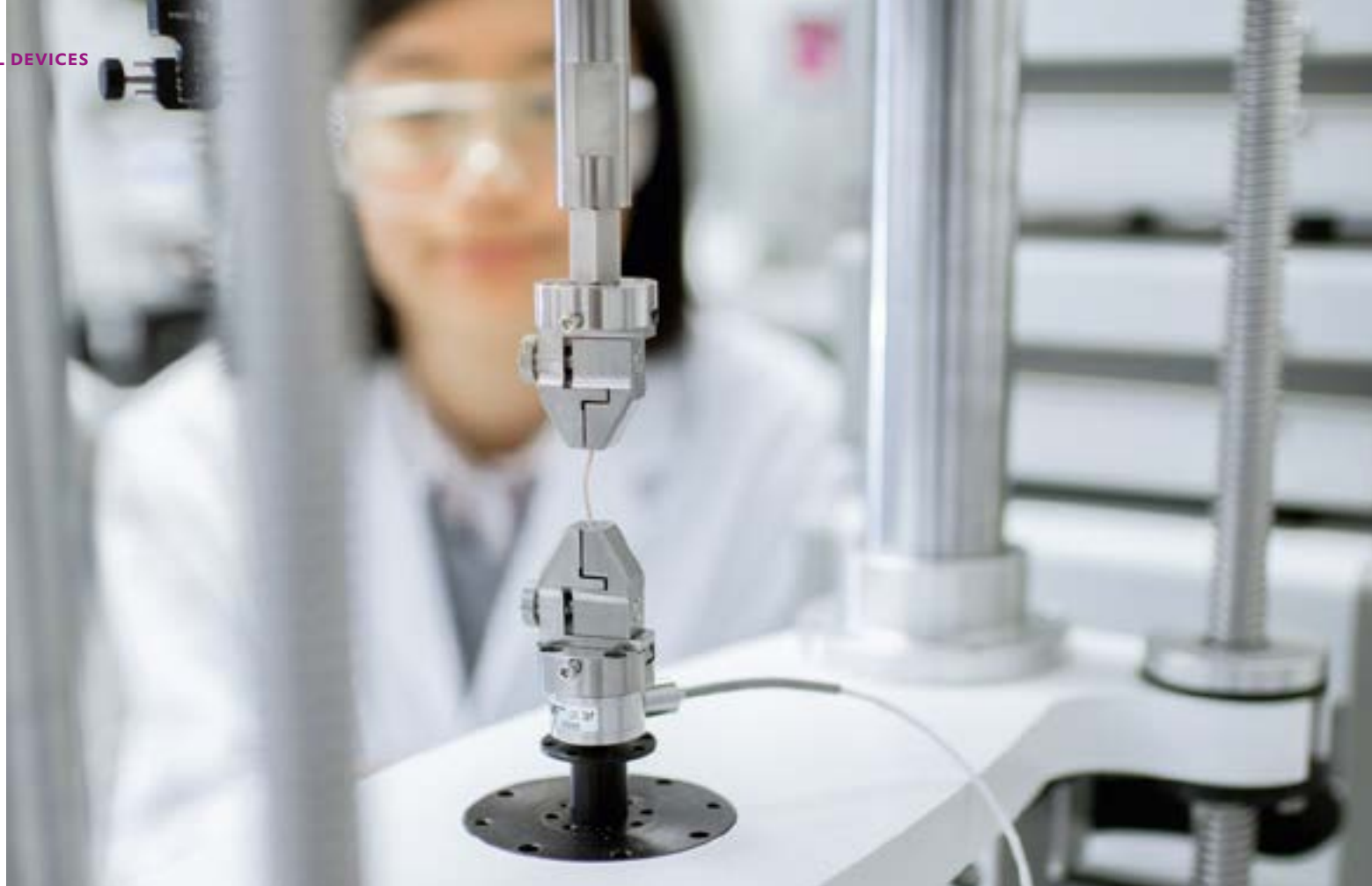
On the test bench: An injection molding prototype made of the newly developed composite material consisting of RESOMER® and hydroxylapatite
