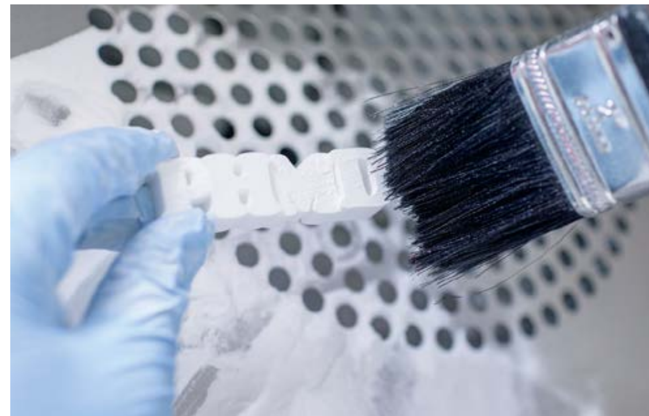
Initial successes with 3D printing: The project house has successfully produced molded parts made of RESOMER® powder through selective laser sintering
