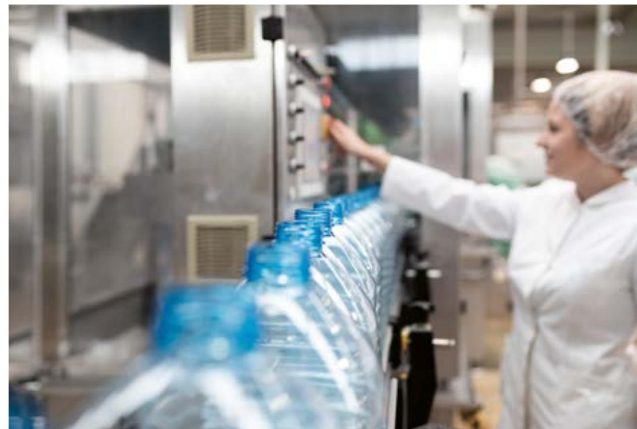
Healthy and durable: In the food industry, PET bottles are sterilized with hydrogen peroxide before being filled
