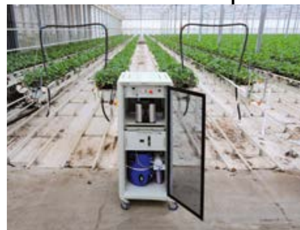
Far from the factory: Distributed H 2 O 2 production in a greenhouse in Denmark
