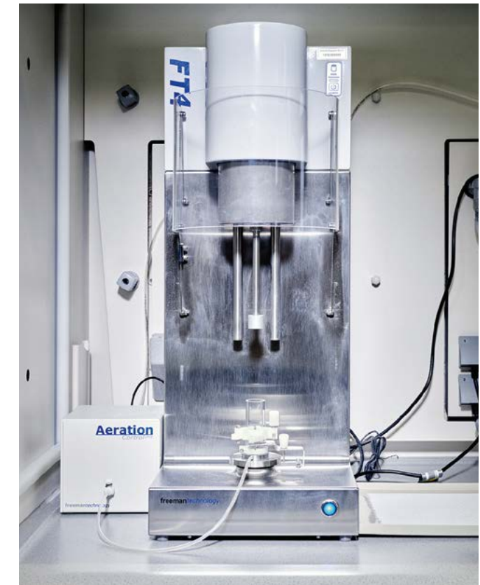
At the Evonik location in Hanau, laboratory assistant Mona Müller monitors the intermediate stage of a catalyst synthesis (left). The researchers use a rheometer to measure the flowability of their powders
