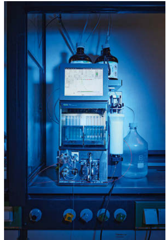
The rPEG lipid is purified by means of chromatography
