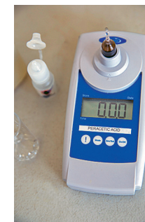
A peracetic acid (PAA) monitor is used to determine the amount of PAA residual remaining in the wastewater
