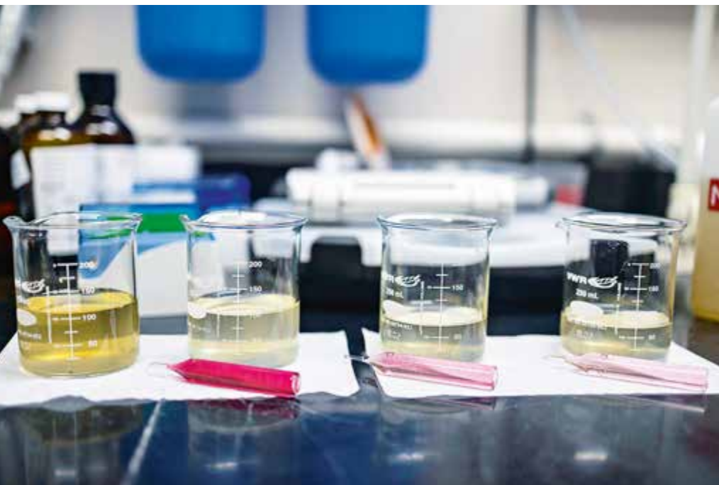
Samples of Memphis wastewater in Evonik's Wolf River plant before (left) and after being disinfected with different concentrations of peracetic acid. As the PAA is consumed by the organic matter and bacteria in the disinfection channels, the wastewater color gets lighter. The pink vials show the residual concentration dropping as the PAA reacts with the contaminants
